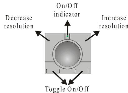
**Toggle On/Off:** The trackerball can be toggled ON or OFF with both keys. When the trackerball is active, the **On/Off indicator** LED will be green (only on new controllers).
